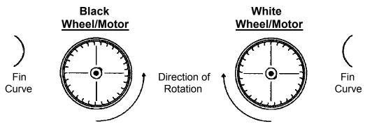
When they are new, you may wish to scratch a "B" into the metal on the back of the black blower wheel and a "W" into the back of the white blower wheel because, after a period of time, the grease and cleaning may obliterate the paint. **Take care to always keep the motors and wheels in their proper locations!** Placing a blower wheel and/or motor in the wrong location may cause the motor to overheat and prematurely burn out. Your Vent-A-Hood will also become noisy and won't ventilate properly.
