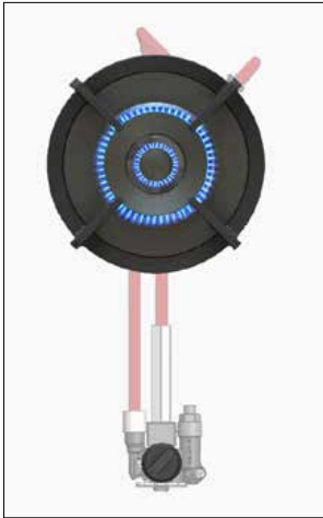
Control knob at the half open position: Gas supply fully open. Both rings are activated.
